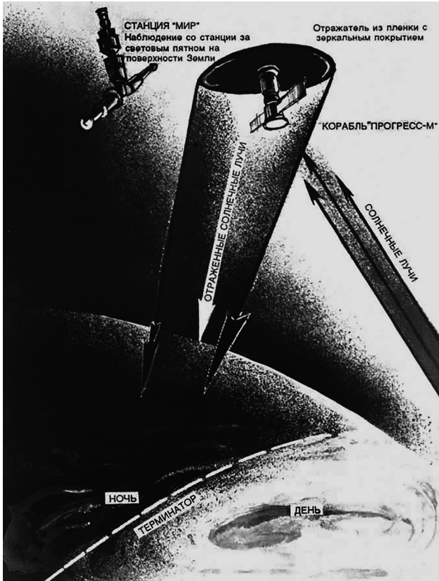
a. Conceptual drawing of the functioning of znatya
