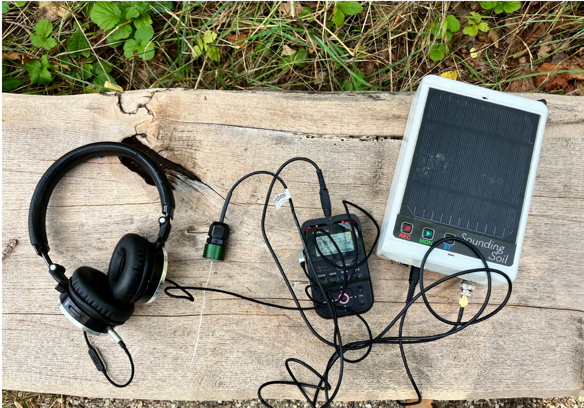
The Sounding Soil kit, plus my own recorder. Using my own recorder with a line in/line out cable enabled me to record directly onto my own machine for any amount of time. The probe for the microphone is present in this photo, it was extremely delicate and I broke the first one I borrowed.
